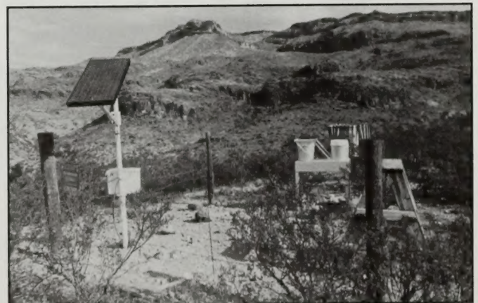
The Oliver Knoll atmospheric deposition monitoring station is part of a nationwide network that measures the acidity and particulate content of precipitation.
